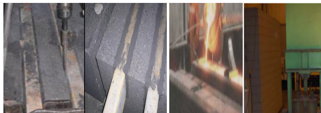
Figure 1 Cathode blocks with current supply sealing using carbon mass (a) and cast iron casting (b)
